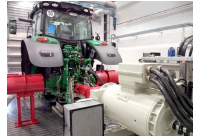
The acid test: PTO test stand at John Deere. A frequency converter from VEM provides for fast implementation of the control commands issued to the test stand. Photo: Karlheinz Bitsch, John Deere Werke
