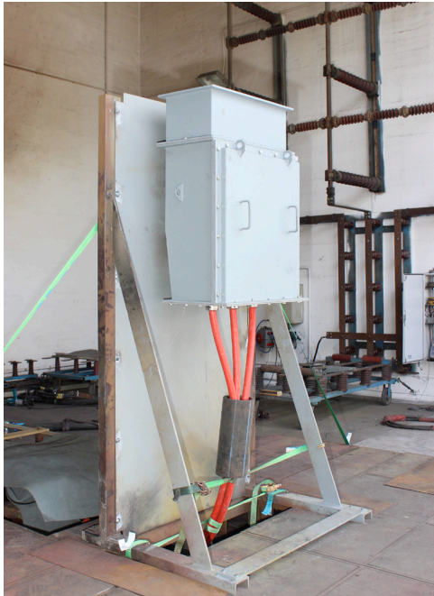
Preparations for an arc flashover test at the German High-Power Test Laboratory (IPH)
