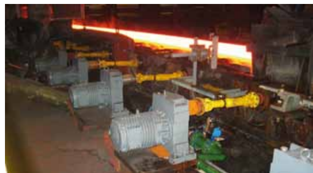
Delay table with S141-1A ARG 160L 4, M_{max}=1039 Nm
