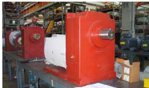
Roller table version, SG200 ARG 200L 8, M_{max}= 1655 Nm
