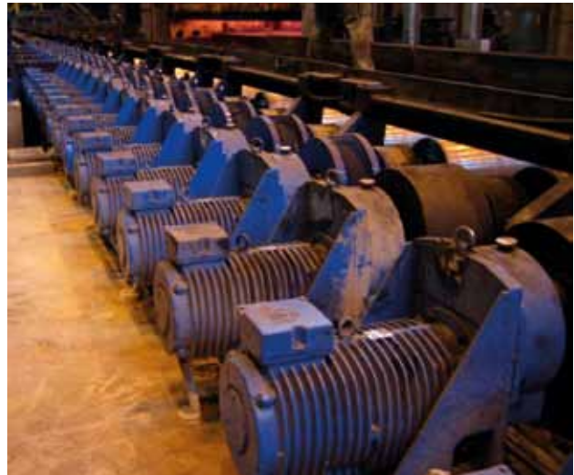
Furnace table with ARG 200L 12, M_{max}=1888 Nm
