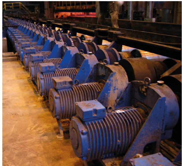
Figure 4: Furnace table with ARG 200L 12, M_{max} = 1888 \text{ Nm}
