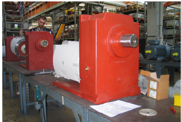
Figure 5: Roller table version, SG200 ARG 200L 8, M_{max} = 1655 \text{ Nm}
