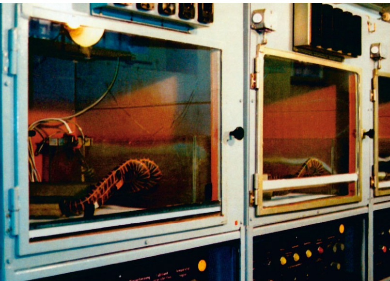
Figure 2: Test facilities for the thermal evaluation of insulation systems
