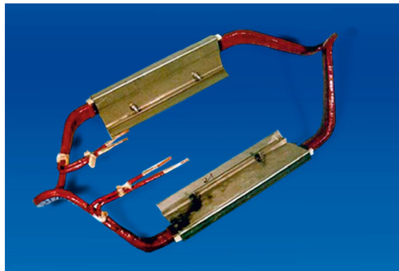
Figure 1: Test object for the determination of long-term heat resistance
