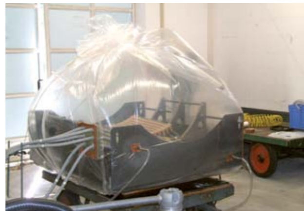
Figure 1.4: Impulse voltage test on a winding model under gas (photo: PTB Braunschweig)
