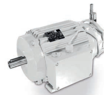
Brake motor in special rail version B210 U 100 LX4, with mechanical brake release, 4.0 kW, S2 10 min
