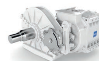
Locomotive drive with asynchronous traction motor with forced ventilation, 1400 kW
